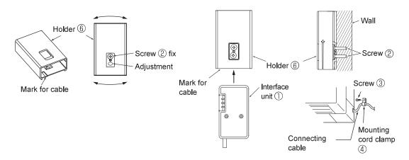
When mounting on the outer side of indoor unit
